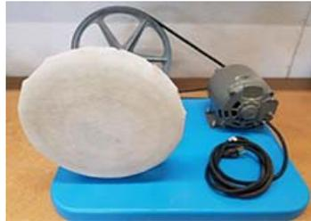
Richardson Buffer – ½ hp 120 vac motor. 12-inch leather buffing disc. \$345.00
